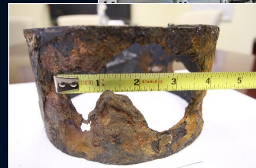
Fire Suppression Lead-in Line Corrosion
