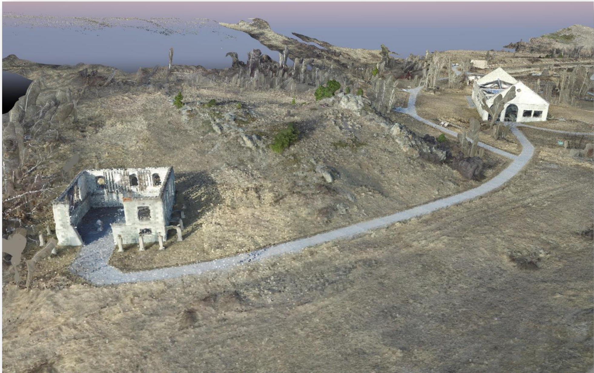
Historic site 3D modeling using UAV in flood-prone area (Leitch Collieries Provincial Historic Site)
