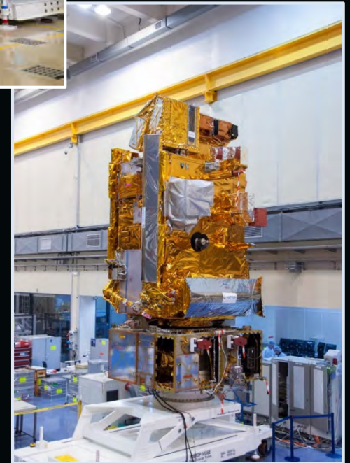
Meteorological Operational Satellite-C (MetOp-C) is the next (and last) in a series of three weather satellites from the ESA and EUMETSAT. Under Interagency agreements with NOAA, NASA (GSFC) is providing four POES heritage instruments AMSU-1, AMSU-2, AVHRR/3, and SEM. Launched: November 7, 2018
